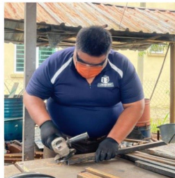
Figure 3.9 Scraping sharp iron after cutting with a grinder
