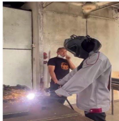
Figure 3.10 Join metal with welding method
