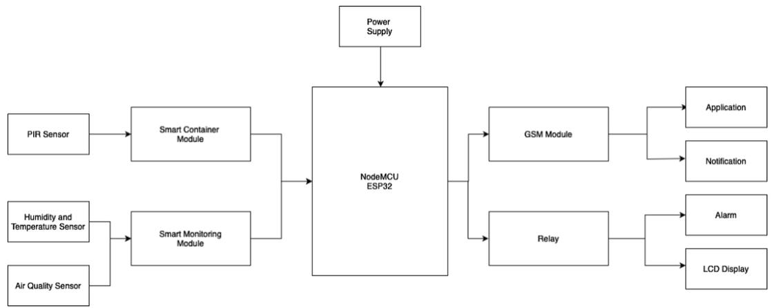
**Figure 1:** Architecture Diagram of IoT-Based Smart Kitchen
