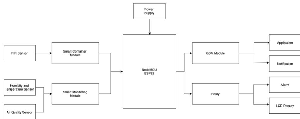
**Figure 3.2.1:** Block Diagram of IoT-Based Smart Kitchen
