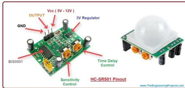
HC-SR501 is an automatic control module based on infrared technology which has high sensitivity and security and works under the extra low voltage mode. It is a common sight that the module is applied in a range of automatic sensing electronic equipment, especially in mechanical control products powered by a dry battery.
