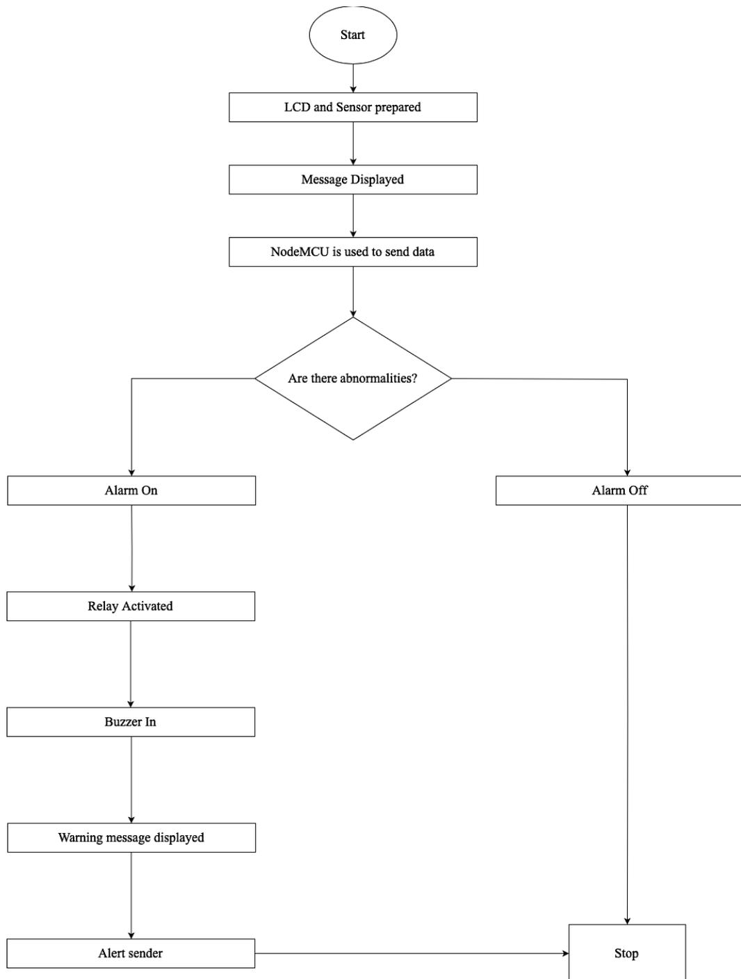
**Figure 3.4.1:** Flowchart of the System of IoT- Based Smart Kitchen Project.
