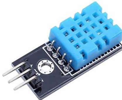
An essential, extremely affordable digital temperature and humidity sensor is the DHT11. It measures the humidity in the air using a thermistor and a capacitive humidity sensor, and it outputs a digital signal on the data pin (no analogue input pins needed). Although it is easy to operate, data collection requires precise timing. When utilising the Adafruit library, sensor readings may be up to 2 seconds old because it can only get new data once every 2 seconds.
