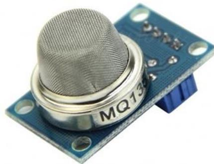
MQ-135 Gas sensors are utilised in air quality control systems and are appropriate for NH<sub>3</sub>, NO<sub>x</sub>, Alcohol, Benzene, Smoke, and CO<sub>2</sub> detection or measurement. When one must detect one gas, the MQ-135 sensor module's built-in Digital Pin allows it to function without a microcontroller. The analogue pin must measure gases in parts per million (PPM). The analogue pin can be utilised with the most popular microcontrollers because it is TTL driven and operates on 5V.
