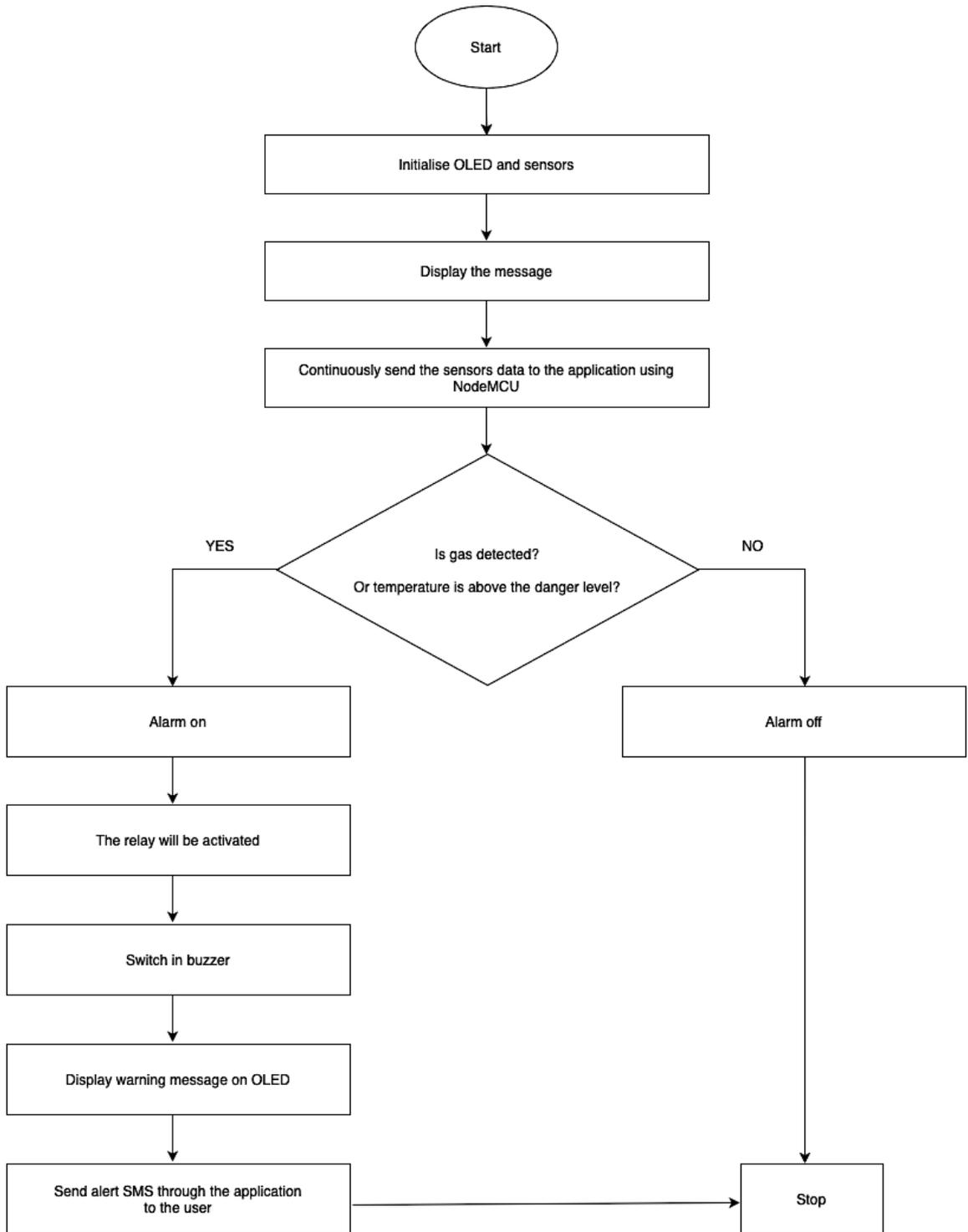
**Figure 3.2.2:** Flowchart of operation for IoT-Based Smart Kitchen
