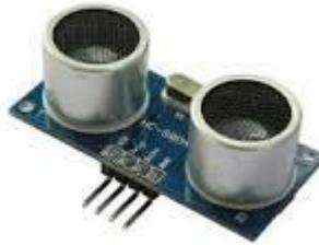
An ultrasonic sensor is an instrument that measures the distance to an object using ultrasonic sound waves. An ultrasonic sensor uses a transducer to send and receive ultrasonic pulses that relay back information about an object's proximity.
