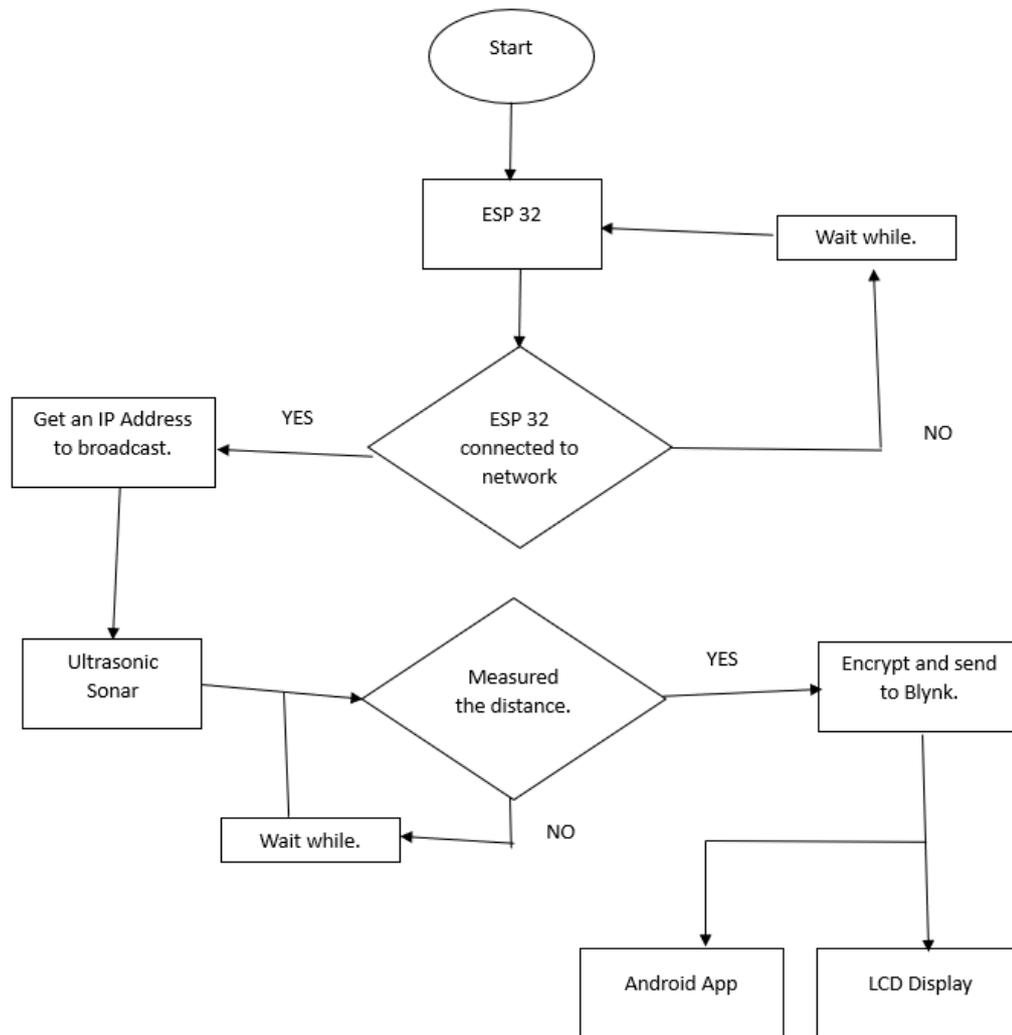
Figure 3.1: Flow chart of IOT laser meters for measuring Distance and depth
