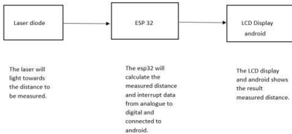
Figure 3.1 Block Diagram
