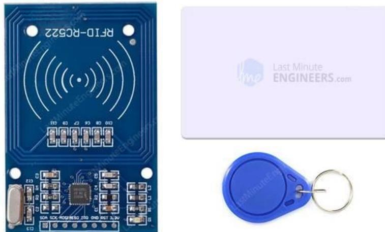
The RC522 is a 13.56MHz RFID module that is based on the MFRC522 controller from NXP semiconductors. The module can supports I2C, SPI and UART and normally is shipped with a RFID card and key fob. It is commonly used in attendance systems and other person/object identification applications.
