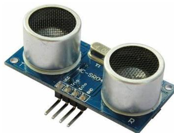
An ultrasonic sensor is an instrument that measures the distance to an object using ultrasonic sound waves.
