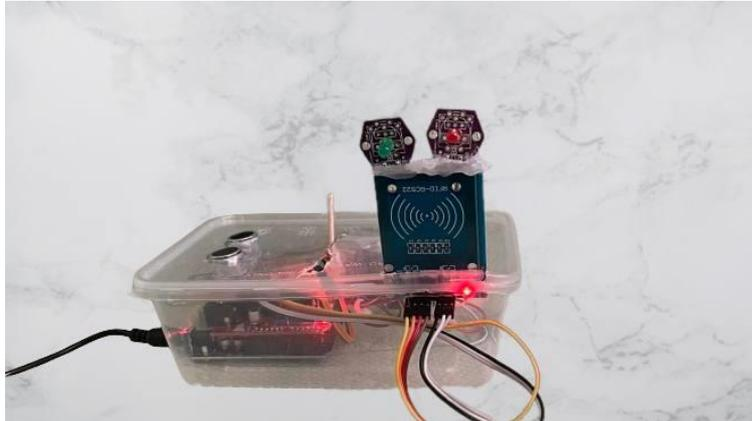
The below diagram shows the status of the parking zone when the auditor scan on the RFID reader using the correct card, the green LED will light up and the barrier will go down
