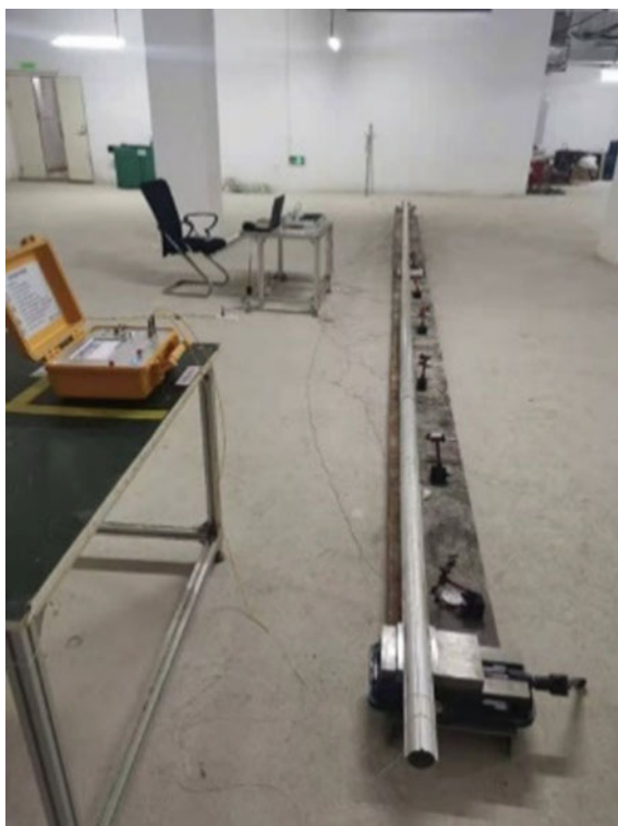
Fig. 7 Schematic diagram of fiber Bragg grating inclinometer
