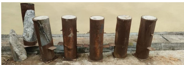
Fig. 8 The steel pipes after test
