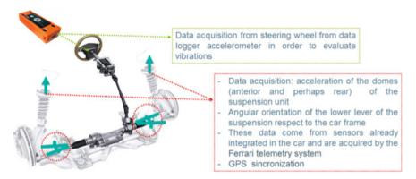
Fig. 7.5 Data acquisition from the steering line
