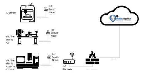
Fig. 5.13 Schema of the IoT sensor node usage
