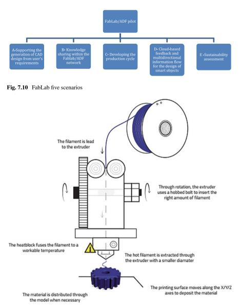
**Fig. 7.11** Schematic representation of fused deposition modeling process. (Copyright BCN3D Technologies, image extracted from the User manual BCN3D+ page 4)
