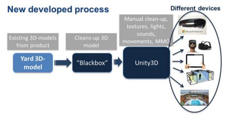
Fig. 7.30 Scheme of new developed process
