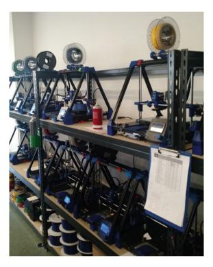
Fig. 5.12 3D-printers making 3D-printers components in fundacio CIM
