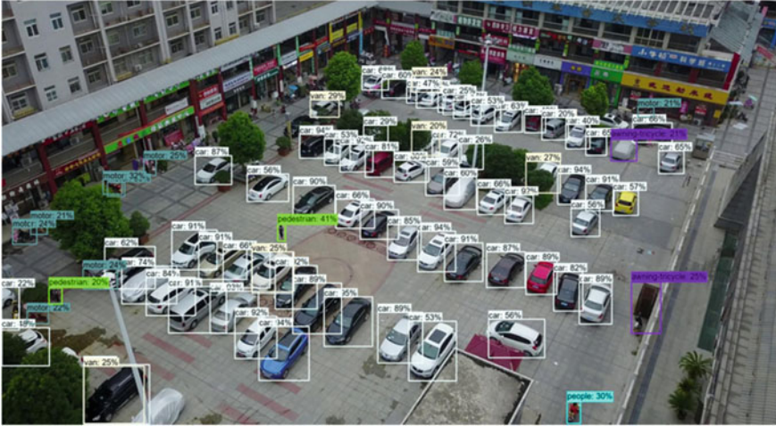
Fig. 5 Vehicle detection results of YOLO on the VisDrone dataset
