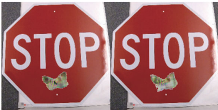
Fig. 3 Adversarial patch attack examples that made the road sign classifier recognize them as “Speed Limit 80” [41]
