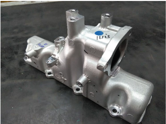
Fig. 2 Manifold, Source Tapukara, Rajasthan
