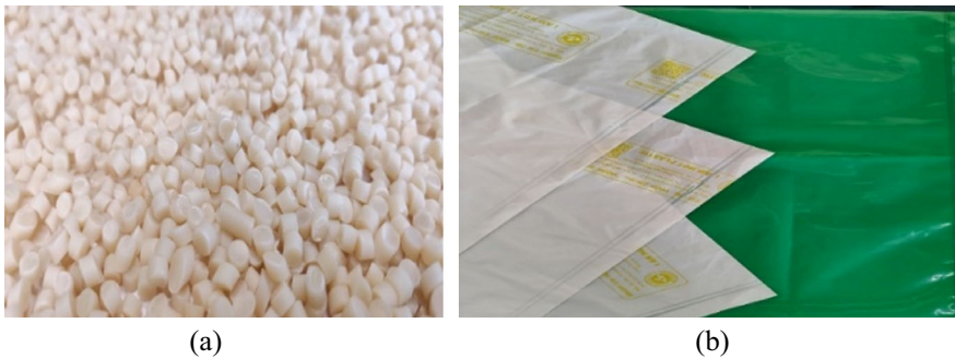
Fig. 2 a Granules of biodegradable plastic b Bio-degradable plastic-bags manufactured from granules
