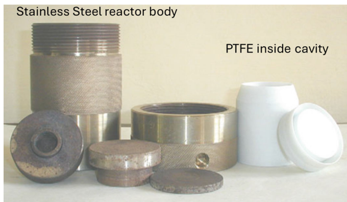
Fig. 10 A general-purpose autoclave reactor. The hydro/solvo-thermal reaction occurs inside the PTFE cavity [57]
