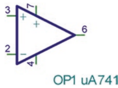
Figure 9-1. The Standard Symbol for the Opamp
