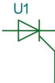
Figure 3-1. The Basic Symbol for the SCR
