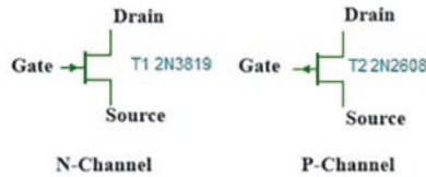
Figure 7-1. The Symbols for the Two Types of JFETS
