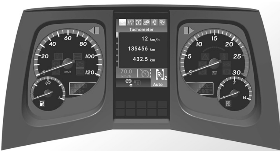
Fig. 1.9 Main instrument panel in a long-distance haul truck. The two large, round gauges show vehicle speed (left) and engine speed (right). The smaller round gauge on the left shows the fill level in the fuel tank, while the fill level of AdBlue or DEF is displayed in the smaller round gauge on the right . In the center is a LCD display in which many digital menus can be called up. (Illustration: Daimler)
