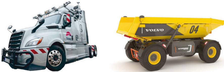
Fig. 4.6 Left: Prototype for autonomous driving based on an established long-haul tractor vehicle with comfortable cab. Right: Prototype for a tipper truck without a cab. As there is no cab, the dimensions of the autonomous vehicle are difficult to judge: this is a tipper with a 15 t haulage capacity. (Photos: Left: Daimler, right: Volvo Construction Equipment)
