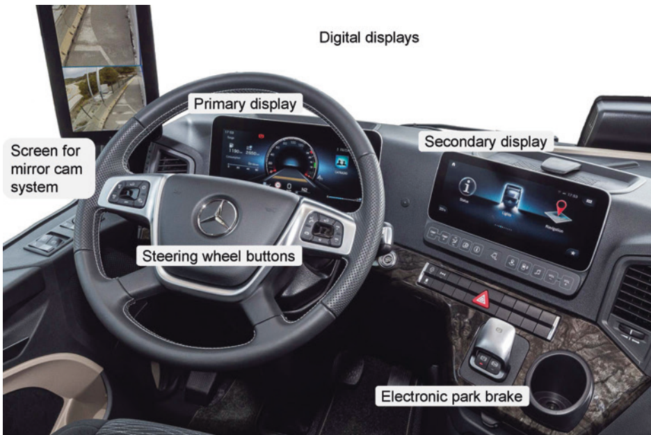
Fig. 1.8 Driver cockpit with two fully digital displays. (Photo: Daimler)
