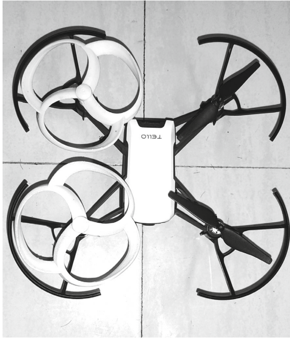
Fig. 9.17 Toroidal propellers and normal propellers mounted on Tello drone
