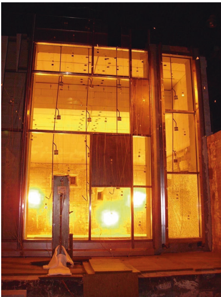
Fig. 13.19 Sample EN 1364–4 fire test [202] (Courtesy of Efectis)
