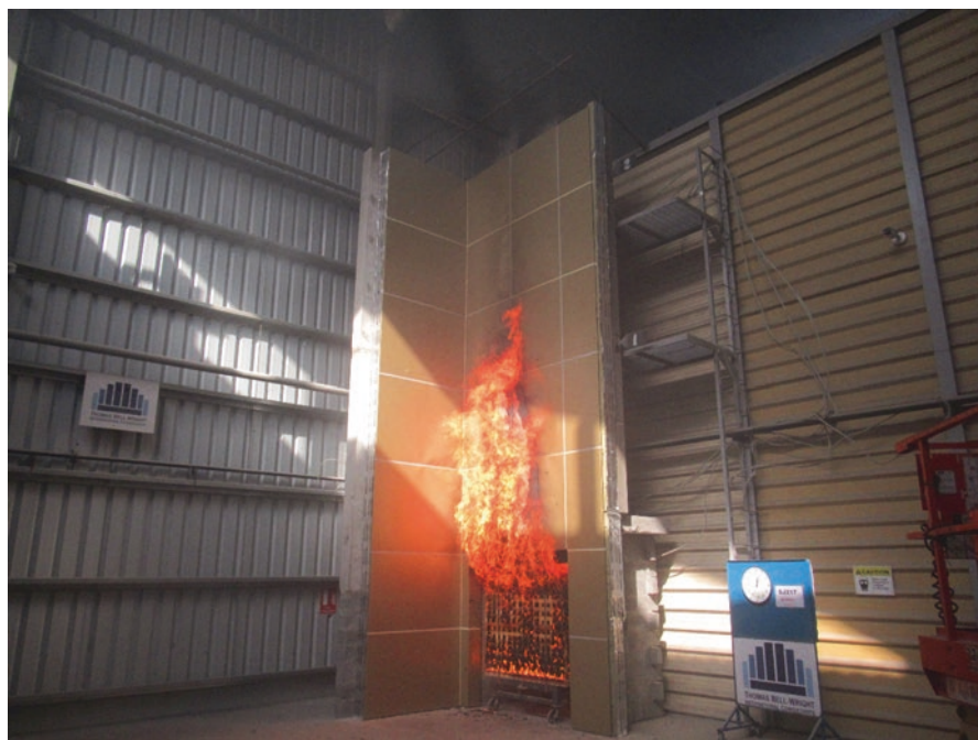
Fig. 13.21 Sample BS 8414 fire rest (Courtesy of Thomas Bell-Wright International Consultants)
