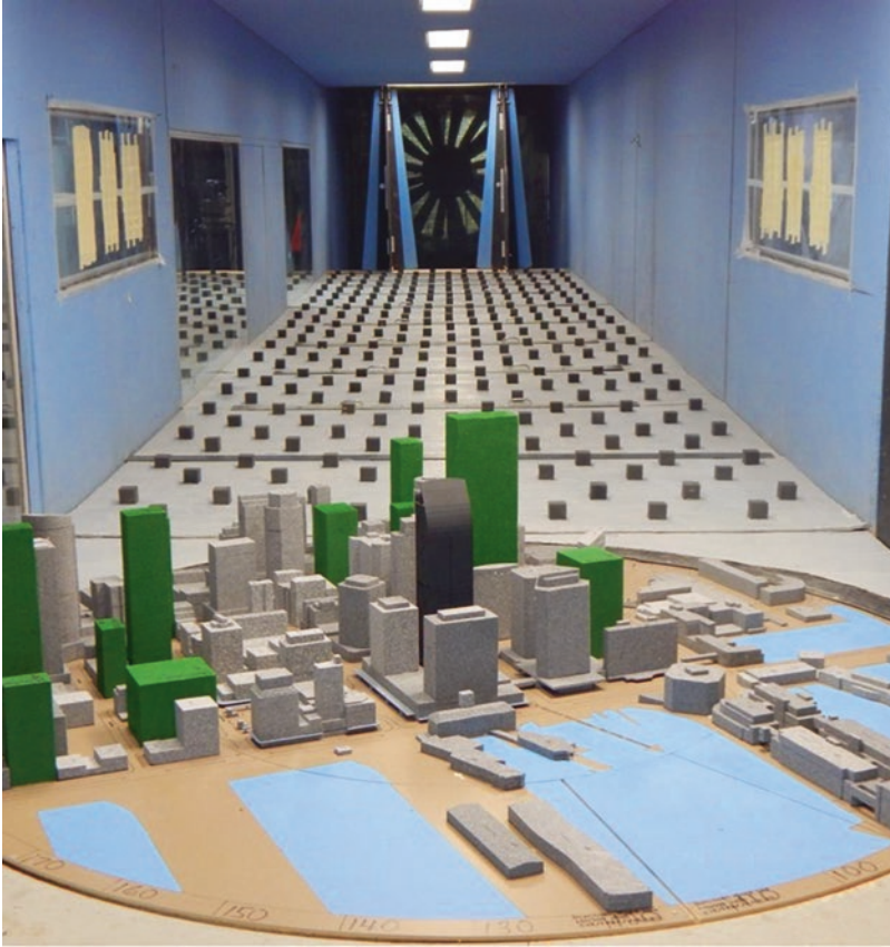
Fig. 16.4 Wind Tunnel Testing of a Tall Building in Auckland. Courtesy of Rowan, William, Davies & Irwin, Inc.
