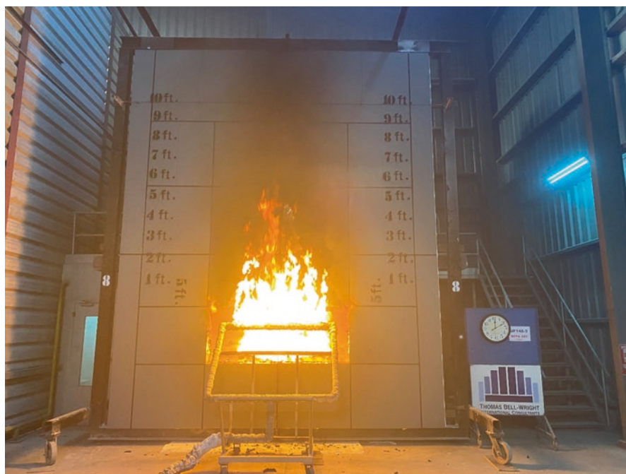
Fig. 13.20 Sample NFPA 285 fire test (Courtesy of Thomas Bell-Wright International Consultants)
