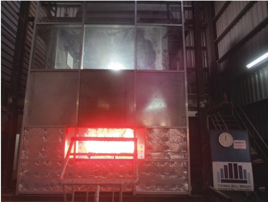
Fig. 13.18 Sample ASTM E2307 [201] fire test (Courtesy of Thomas Bell-Wright International Consultants)
