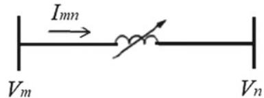
**Fig. 2** TCSC in capacitive mode
