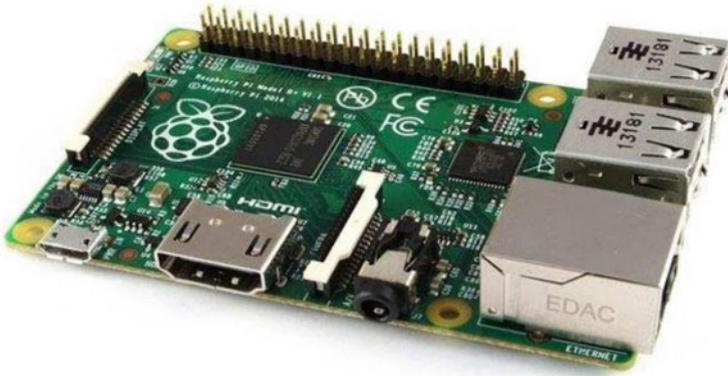
Fig. 2 Raspberry Pi single-board computer
