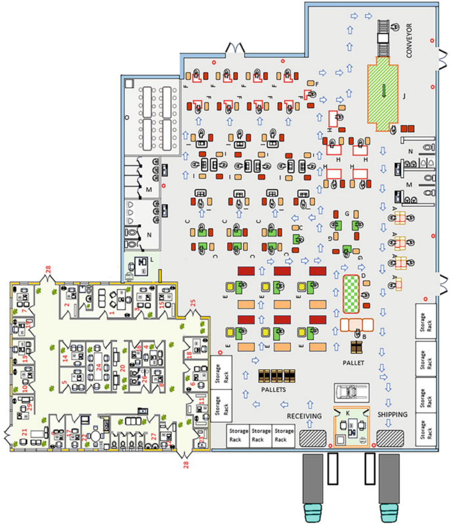
Fig. 12.14 Final plant layout
