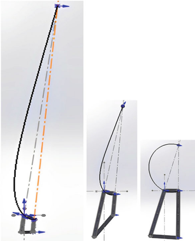
Fig. 6 Represents the simplification of the 4-bar mechanisms of commercial prostheses and the evolution of the ICR
