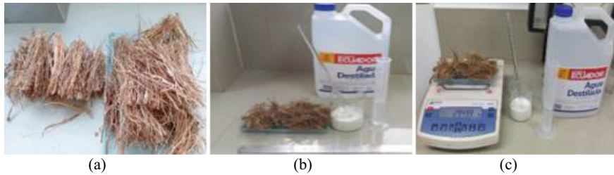
Fig. 2 Materials and equipment: a coconut fiber, b natural rubber latex, test tube, agitation rod, beaker, distilled water, c scale
