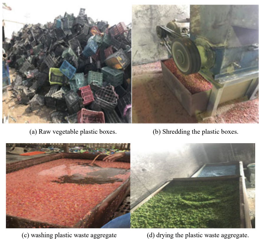
Fig. 1. a Raw vegetable plastic boxes. b Shredding the plastic boxes. c Washing plastic waste aggregate. d Drying the plastic waste aggregate
