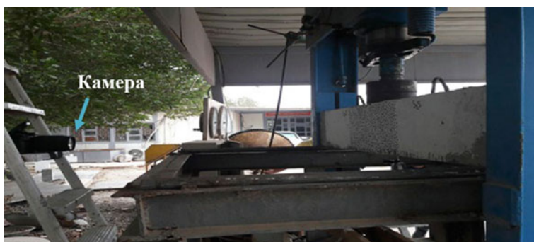
Fig. 3 Experimental setup of digital image correlation technique
