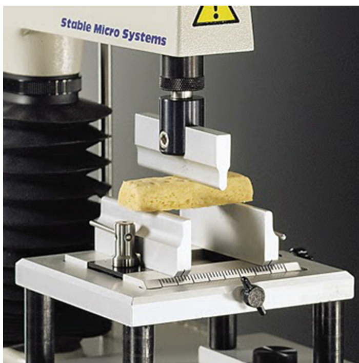
Fig. 2. 3-point bending test on biscuits [26].
