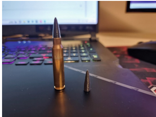
Fig. 6. 3D printed projectile for 5.56 × 45 mm bullet.
