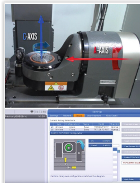
Fig. 2. Defining rotary axes on the HAAS control unit [26]
