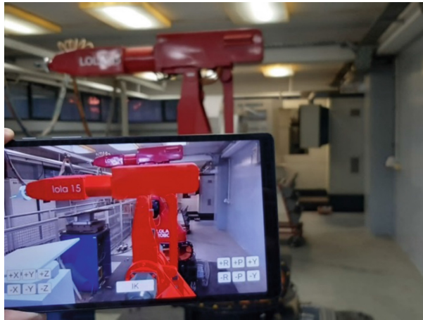
Fig. 3. AR integration of robot model in the real-world laboratory environment for simulation and verification of programmed robot motions
