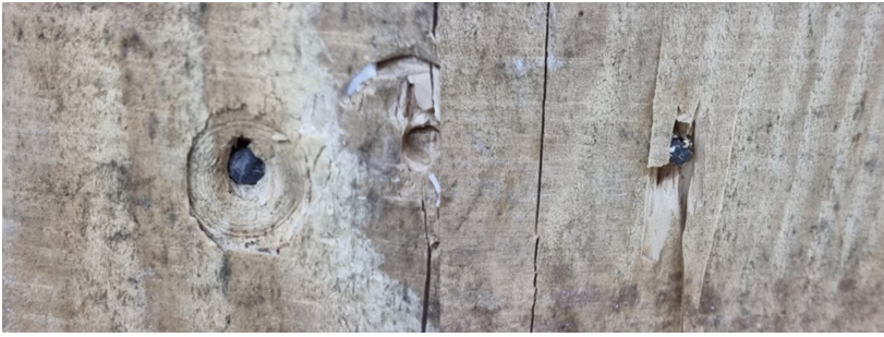
Fig. 9. Penetration of 3D printed polymer projectile into the wooden board [57].
