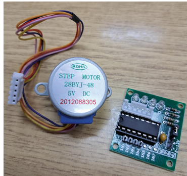
Fig. 1. A stepper motor 28BYJ-48 (on the left) with motor driver TI ULN2003AN (on the right).
