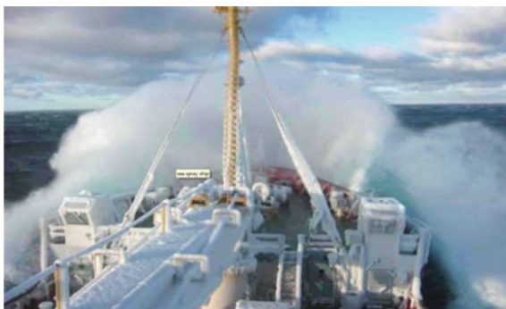
Fig. 5.3 Vessel–wave interaction and resulting sea spray icing on the deck [17]
