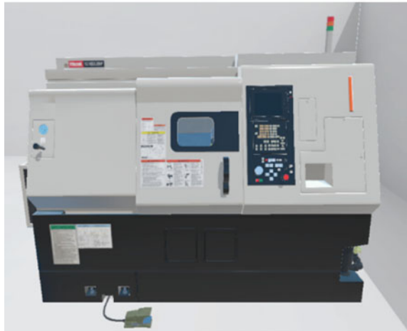
(b) Virtual CNC Turning machine
