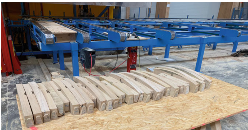
Fig. 7 Dovetail joined parts, produced using a Hundegger K2i industry machine
