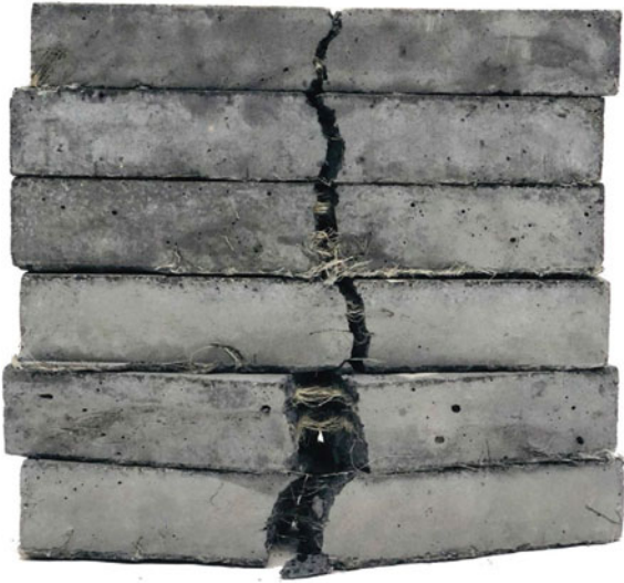
Fig. 14 Comparison of the flexural strength of BCMs and BGCs of specimens with and without hemp fibre
