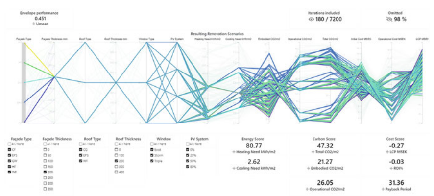
Fig. 14 Optimal roof thickness is 200 mm
