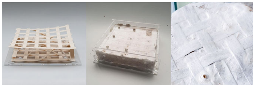
Fig. 11 The HOME project investigated the combination of additively manufactured timber 3d lattices in combination with bio-growth of mycelium, producing a novel reinforced biomaterial, that is fully compostable
