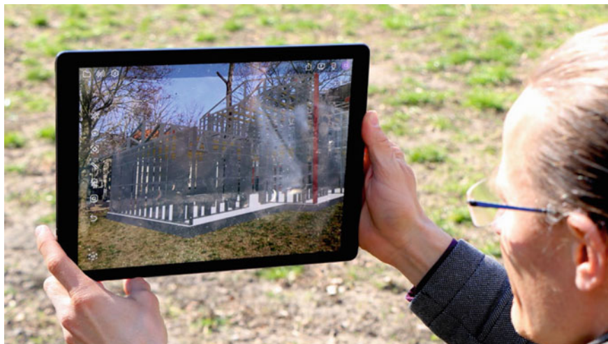
Fig. 11 Tablet used to visualize the dwelling in the lot (non-immersive AR)
