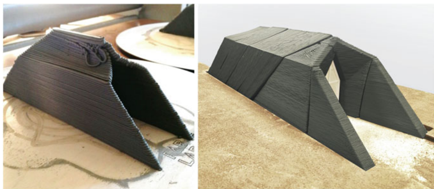
Fig. 12 The prototypes with different slicing methods: horizontal and 45° layering
