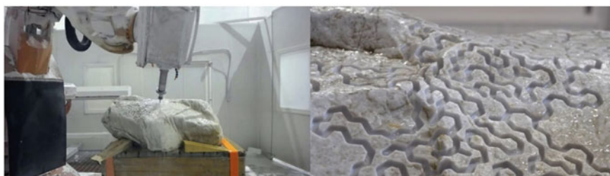
Fig. 11 Left—Fabrication using 7 axis milling, Right—Milling details
