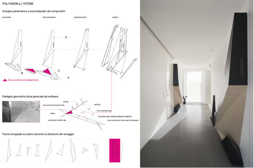
Fig. 3 The diagram illustrates the phases of recursive computation for the generation of the executive 3D digital twin of the guestrooms' totems
