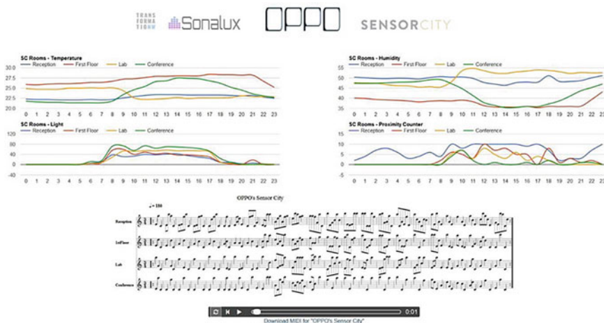
Fig. 2 OPPO: the web-based version translating live data from four sensors in four different rooms onto a musical score
