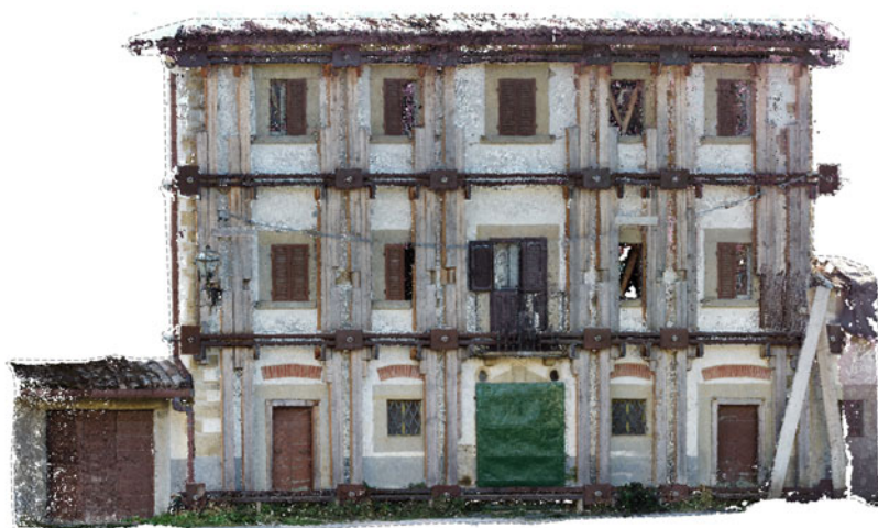
Facade survey point cloud: N.points 1701997
