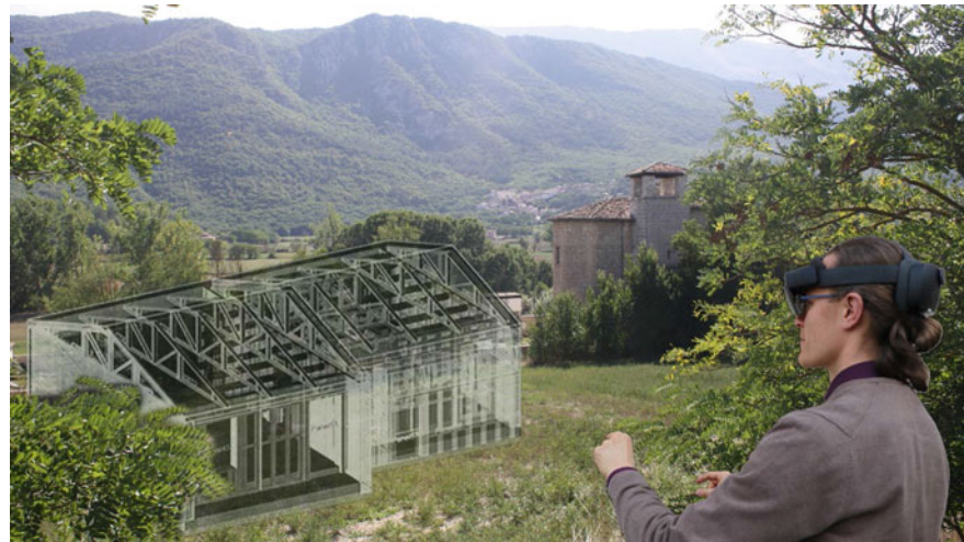
Fig. 10 Hololens 2 used to visualize the dwelling in the lot (immersive AR)
