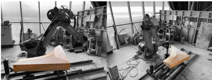
Fig. 17 Laminated timber prototypes produced using hybrid methods
