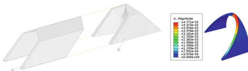
Fig. 11 Components of the nubian vault prototype and FEM printability simulation
