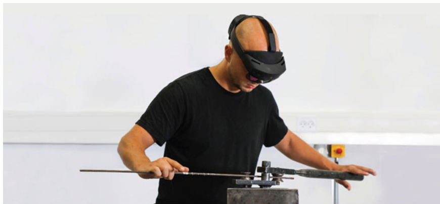
Fig. 10 Three-dimensional rebar bending in MR
