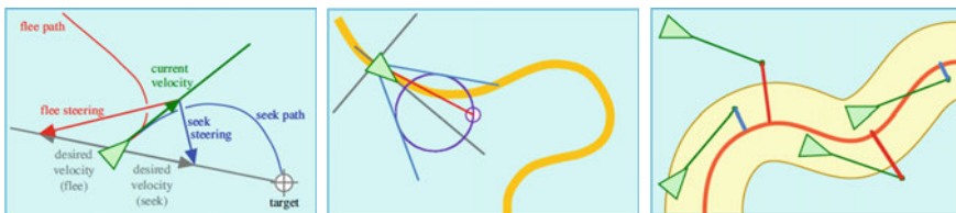
Fig. 12 Reynolds steering behaviour diagram. Left, Seek & Flee behaviours. Centre, Wander behaviour. Right, Path following (Reynolds, 1999)
