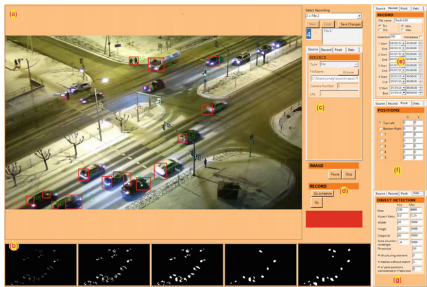
Fig. 4 Computer application, in real time, for processing the images of the video cameras
