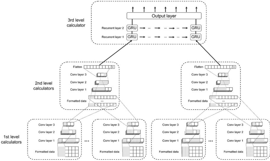
**Fig. 1.** The structure of hierarchical neural network model
