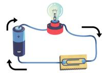
A dry cell provides the 'push' needed for electrons to flow in the loop. These electrons are already present in the wires. When these electrons pass through a load or a receiver, electrical energy can change into other forms, such as
