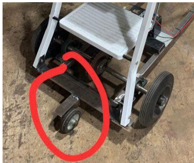
Figure 3.12: The part that has been added stabilize the ladder.
