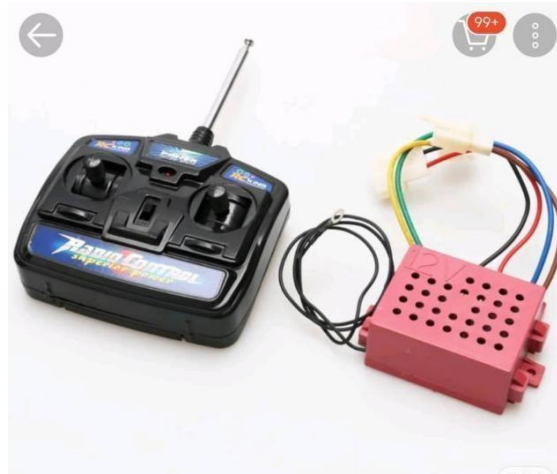
Figure 3.9.7 : 27Mhz 4ch Remote Controller
