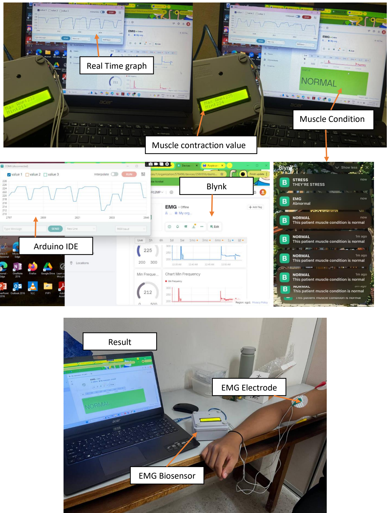
Figure 4.1 EMG Biosensor for Athlete by using ESP32 with IoT Application
